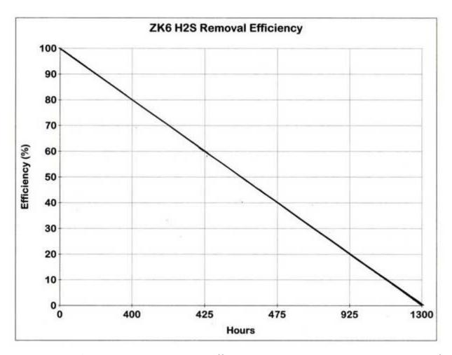
The chart above illustrates the ZK6 efficiency when challenged with 50 ppm of hydrogen sulfide. The media performed in excess of 1,300 hours before being expended.
